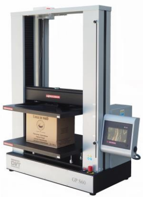
DVT GP D S60 N BOX CRUSH TESTER
